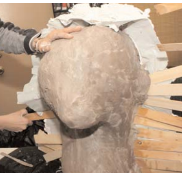
Removing tape and shims to prepare for second mould piece.
