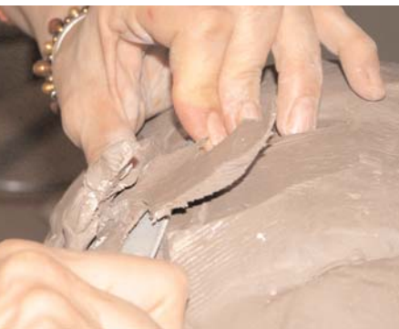
Cut and smooth the rough clay mould lines.
