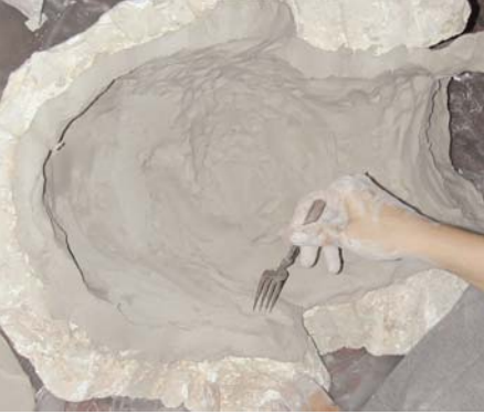
Poke holes for better drying and firing of the clay.
