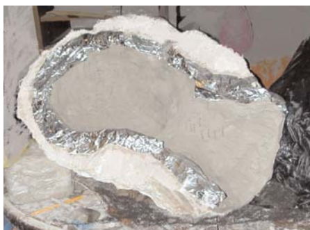
Keep edges moist while the inner clay stiffens after pressing clay into the mould.
